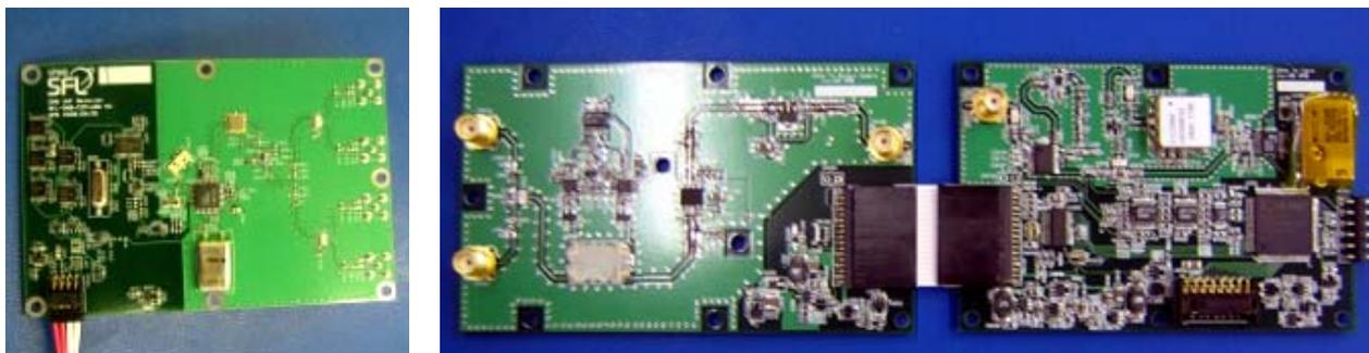
Figure 9: UHF receiver (left) and S-Band transmitter (right).
