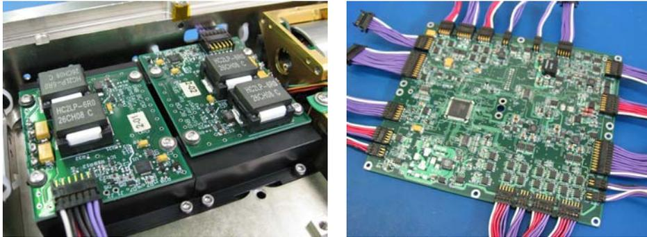
Figure 8: BCDR (left) and Power Distribution Unit (right).
