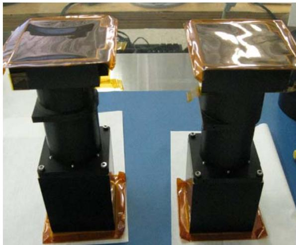
**Figure 14: The BRITE Telescope.**
