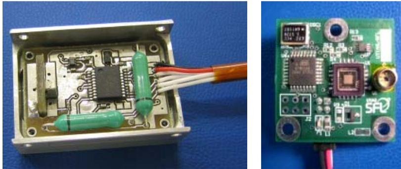
Figure 10: Magnetometer (left) and Fine Sun Sensor (right).
