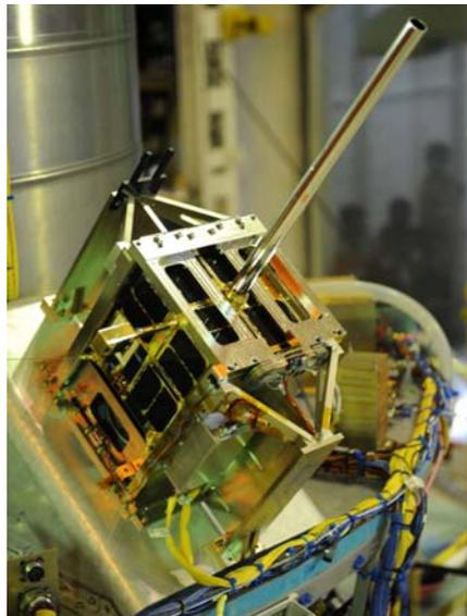
Figure 15: AISSat-1 Launch Configuration, showing the 162 MHz payload antenna.
